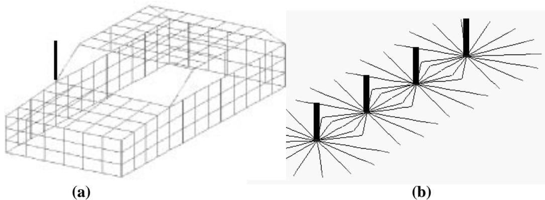
**Fig.2.2:** The segmentation of (a) a wire antenna over a car, (b) four vertical monopoles with 16 ground screen radials under each
