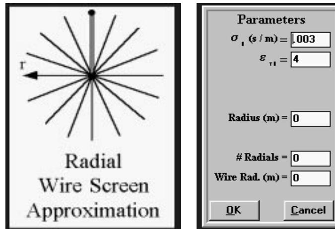
**Fig. 2.3:** Ground screen with radial wires in NEC (NEC calculates approximate equivalent surface impedance for the ground and screen)
