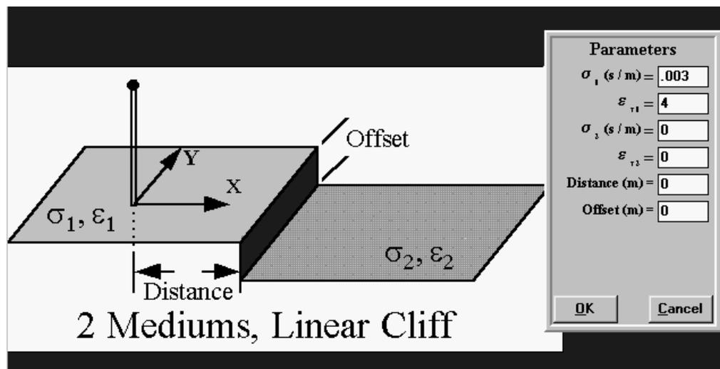
**Fig. 2.4:** Linear cliff modelling and two mediums with parameter specifications in NEC. By using this module, land-sea coupling, beam shooting over a hill towards the sea can be modelled up to a certain extent. The two medium parameters, distance from the antenna to cliff and the cliff's height above sea level are supplied from the table on the right. The antenna must be on the upper medium.
