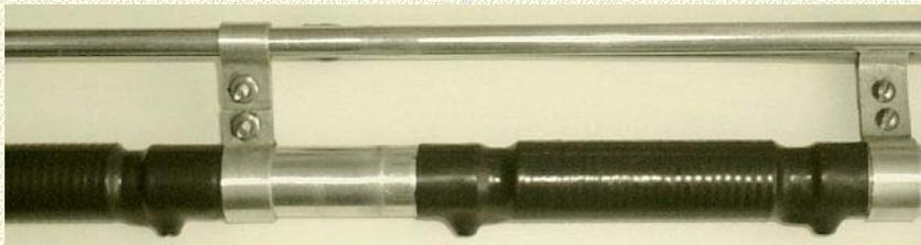
Cleaned and repaired coil
