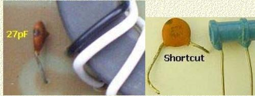
I replaced a shortcut 27 pF cap with 4 × ceramic tube caps in series/parallel.
